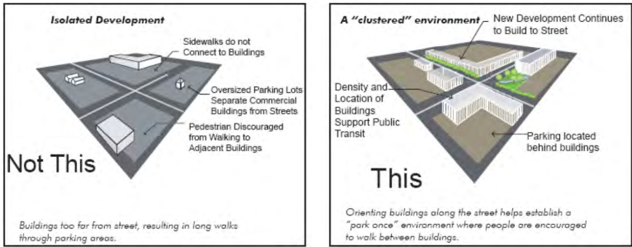
Figure 19.3: Setbacks have a negative effect on safety, walkability and public transport usage of a place. Cluster building entries near nodes, bus stops, etc. to offer a one-stop opportunity to conveniently access a variety of destinations on foot.
